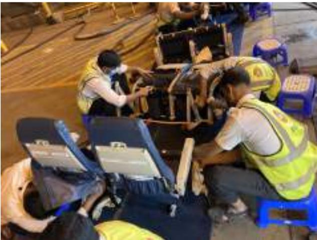
work required to restore the airplane to the flight ready status. A lot of other maintenance measures were taken including installation of protective covers for Engines,
